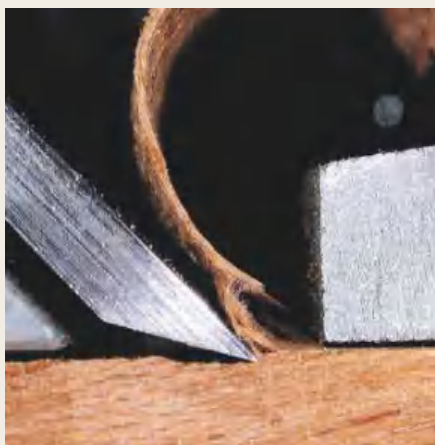
▲ Pic.2 Moving to the right, cutting with the grain, the edge has cleanly severed some fibres while the back face pushed them upwards
